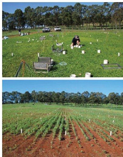
> Figure 5: Field trials and field monitoring of soil greenhouse gas emissions from a biochar field site in northern NSW. Field trials with 0 and 10t/ha poultry biochar (van Zwieten et al., NSW-DII)
